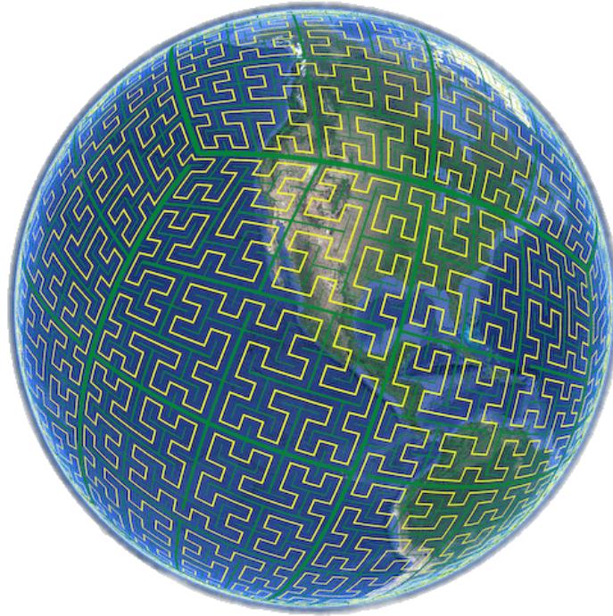
Figure 2.4: Visualization of the space-filling curve used for numbering of cells, Source: [33]
